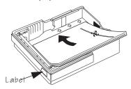
» Note: A label on the cassette shows which paper size to use. Use only that size. As a cassette is inserted in the printer, it sends an identifying signal to the printer's controller board so the printer can
